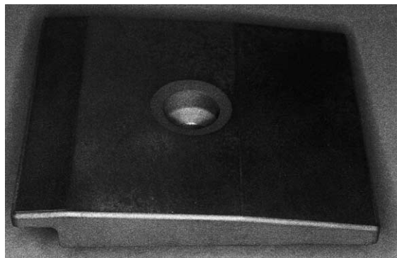
Fig. 2. Optimized tile with trapezoidal shape to reduce the edge power load. The size of a tile is approximately 80 × 80 mm 2 .
